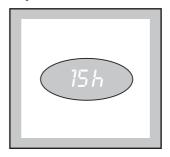
The delay time is displayed for 3 seconds, then the duration of the selected programme reappears. After you have pressed the "**Start/Pause**" button, the delay time value displayed will decrease by units of one hour every hour. When only two hours remain, the display will decrease in 30 minute steps down to zero.
